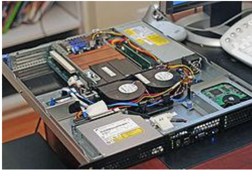
Inside of a Rack unit Server
